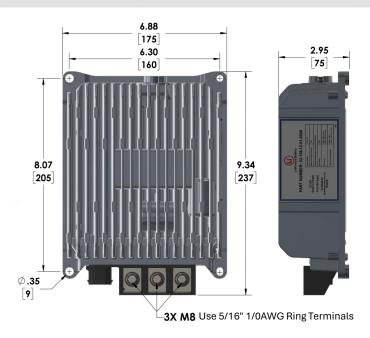
NOTE: DAMAGE TO THE DC-DC WILL OCCUR IF YOU SWAP INPUT AND OUTPUT WIRES, OR IF YOU APPLY REVERSE POLARITY TO THE CONNECTORS. DO NOT OPEN THE DC-DC CASE - THERE IS A RISK OF ELECTRIC SHOCK, AND YOUR WARRANTY MAY BE VOID. CONTACT LITHIONICS BATTERY® FOR A USER INSTALLATION GUIDE & STORAGE PROCEDURES. FOLLOW THEGUIDE TO ENSURE FITNESS OF USE & WARRANTY.
