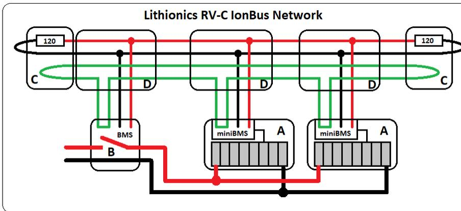
2. **Use one CAN terminator from the customer's CAN network and one IonBus® terminator.** If customer's CAN network spans the distance where Lithionics ESS is at one end and additional CAN equipment is at the other end, it might be convenient to use one IonBus® terminator (C) at the ESS end and one customer's CAN terminator at the other end, see diagram example below.
