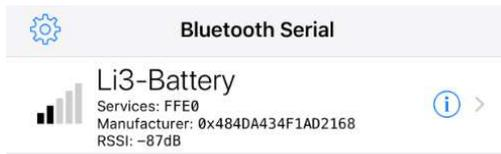
Once the app is installed, open it and connect to the BMS. Typical name of the Bluetooth module is **Li3-Battery**.
