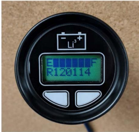
Round Display Pod showing Status Code on the bottom line
